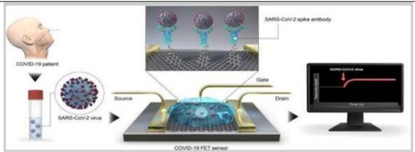
Fig. 9 Systematic process of FET based sensor for COVID-19 detection [2]
